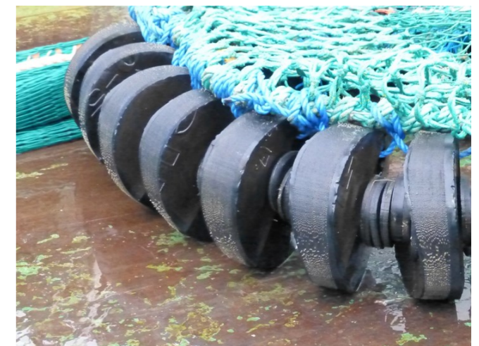
350mm rockhopper gear with belt spacers in between each disc
