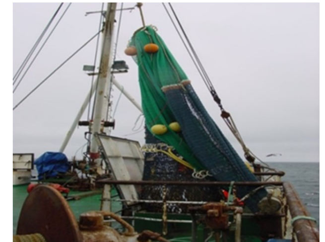
Codend being lifted aboard made from Medium tenacity twine
