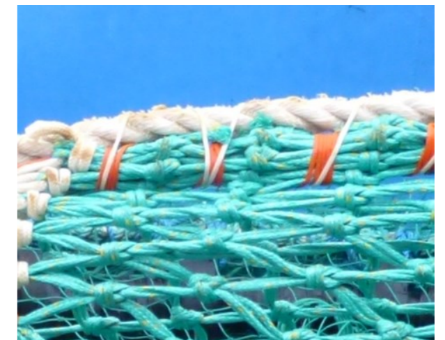
Lestridge made with polypropylene rope
