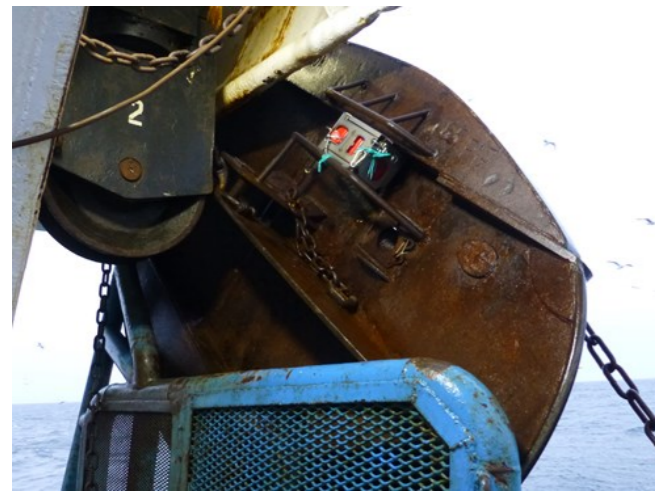
Scanmar distance sensor in its bracket on the starboard trawl door
