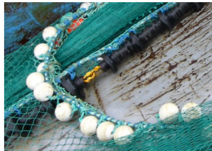
Combination rope headline and footropes
