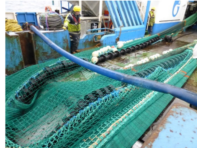
Trawl being hauled aboard RV Scotia – shows different netting panels
